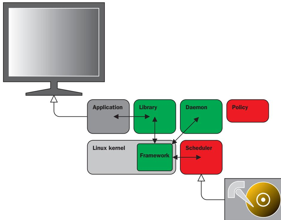
system library that provides access to the ABISS functions. For technical reasons, the functionality to manage the scheduling policy and the scheduling algorithm was separated into two components. A background process (called a daemon in Linux terminology) communicates with the ABISS framework to execute the scheduling policy. Policy settings are provided through a small component (a plugin) that is loaded by the daemon.
